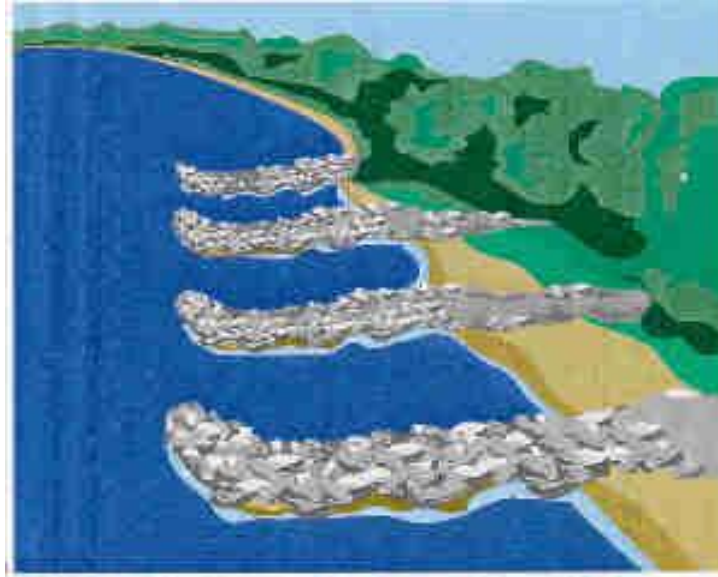
Figure 4-9. Drawing of Wing Dikes Along Bank of River ( Source: USACE, St. Louis District 2005 ).
