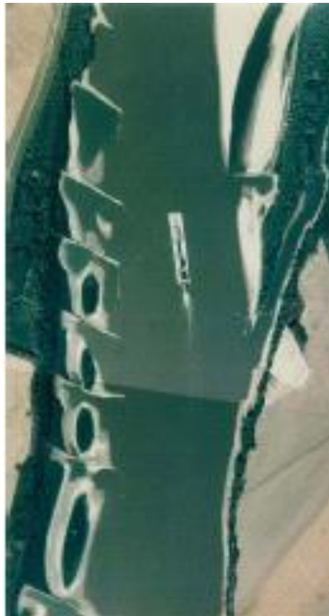
Figure 4-10. Aerial Photograph of Sediment Build Up Behind Notched Wing Dikes ( Source: USACE, St. Louis District 2005 ).
